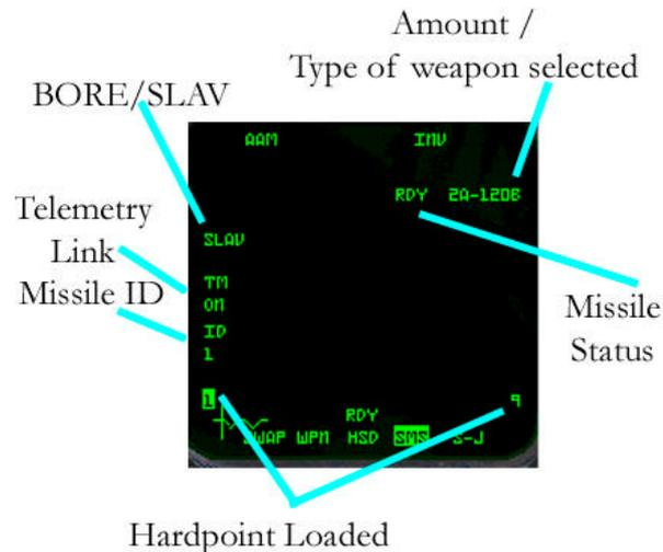
The Amount and type of weapon that are selected appears on the top right hand side of the screen. The number in front of the A-120B is the amount of the missiles that you have loaded. The Missile Status indicates whether the missile is ready to fire (RDY), Safe (SAF), in simulation mode (SIM) or has a problem (MAL). If the status shows MAL then you will be unable to fire it.
