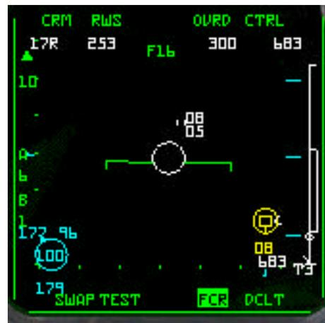
The ASEC will be at its largest when the contact is heading towards you. The chances of successful missile engagements are greater when you are head-on to your target and closure is high.
