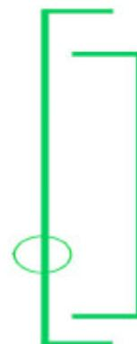
The numbers next to the range indicator are NOT the range. These numbers represent the closure rate of the target in knots. If there is a '-' in front of the number, the target is moving away from you. Finally with the DLZ is the AMRAAM Active Range. This little circle gives you an indication of how far away the AMRAAM will transition from inertial to active tracking. More on this later
