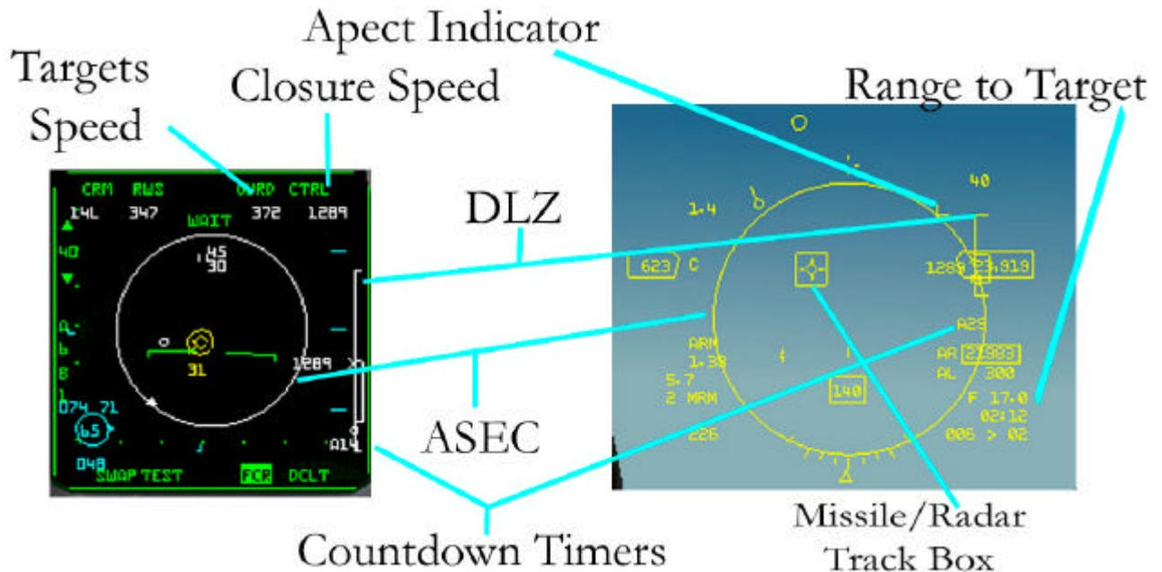
The first indicator that you need to pay attention to is the FCC mode indicator underneath the airspeed on the left. When the AIM-120B is selected the text changes to inform you of this. In this example you can see that the weapon is indicated as MRM (Medium Range Missile). In front of this is the amount indicator, which tells you how many of that weapon you have loaded at that time, in this case two.
