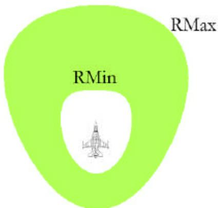
The first thing that needs to be understood when using any air to air missile is the concept of the weapon engagement zone (WEZ). The WEZ is the area around the target where the missile can reach and destroy the target. The diagram to the left shows an example WEZ for a non-maneuvring target. The AIM-120B has a maximum (RMax) and a minimum (RMin) firing range, the diagram represents the area between these two as a green 'doughnut'.
