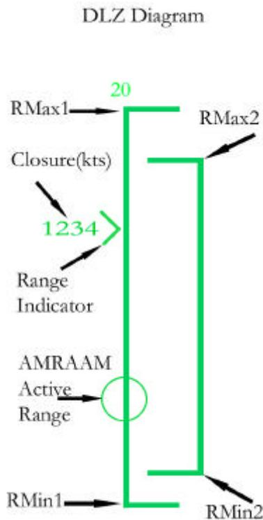
The Dynamic Launch Zone (DLZ) is a set of brackets on the side of the HUD and the Radar screen. The DLZ is comprised of two separate brackets, a distance indicator, and a closure meter. (Note the DLZ will only appear when you have a target selected). The diagram to the left labels the components of the DLZ.
